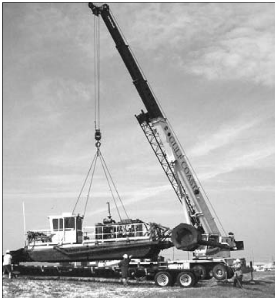
Above, Gulf Coast Crane uses a 75-ton Link-Belt hydraulic crane to lift gasoline tanks into place. Below, a similar crane places a dredge on a trailer for transport.
